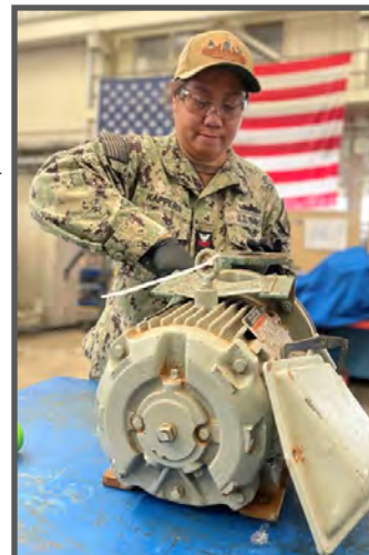
MM1 Anna Kappers works to overhaul and test a VCHT discharge pump on April 8, 2025, at Southwest Regional Maintenance Center. (Photo by MM1 Willy Ann Wray.)
