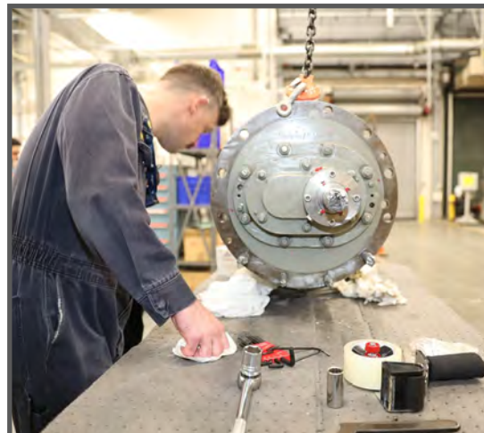
Department Leading Chief Petty Officer MMC (SW) Andrew Huhra completes a visual inspection on the attached lube oil service pump. (Photo by MM2 (SW/AW) Bianca Reiter.)
