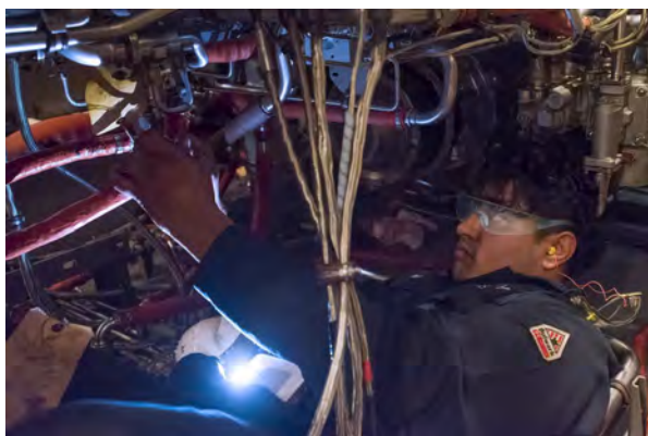
250327-N-GC612-1037, PEARL HARBOR, Hawaii (March 27, 2025) – Gas Turbine Systems Technician (Mechanical) 1st Class Sagar Patel installs a starter to a gas turbine engine on board Arleigh Burke-class guided-missile destroyer USS Hopper (DDG 70) at Joint Base Pearl Harbor-Hickam March 27, 2025. Hopper is at Pearl Harbor Naval Shipyard and Intermediate Maintenance Facility for scheduled maintenance and modernization by Hawaii Regional Maintenance Center. PHNSY & IMF is a field activity of Naval Sea Systems Command and a one-stop regional maintenance center for the Navy's surface ships and submarines. It is the largest industrial employer in the state of Hawaii. Strategically located in the heart of the Pacific, it is the most comprehensive fleet repair and maintenance facility between the U.S. West Coast and the Far East. Its location places it about a week's steaming time closer to potential regional contingencies in the Indo-Pacific. (U.S. Navy photo by Mike Wilson)
