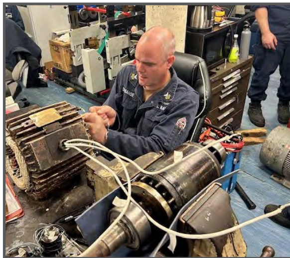
EM1(SW) Marcus Donahoe conducting rewind operations on the exhaust motor for the forward enlisted galley. (Photo by Ramir Pulido.)
