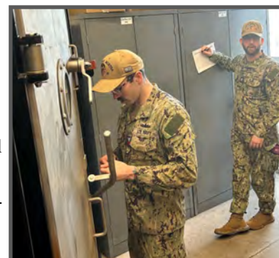
(L-R): HT1(SW/AW) Adam Smerekar of USS John P. Murtha measuring gasket compression on a MAFO Holtkamp Door with shipmate FC3 Joseph Maggiorre recording measurement data.
