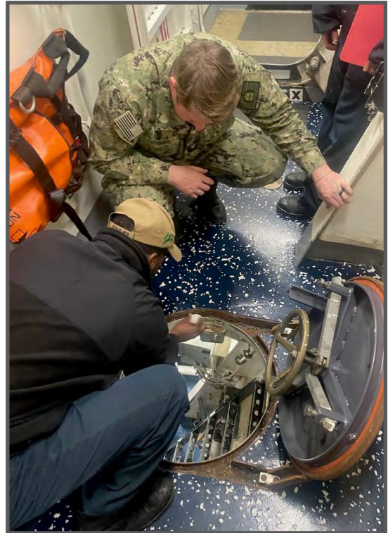
Damage Controlman 3rd Class Christopher Combs, left, supervises a USS LASSEN (DDG 82) Sailor performing a chalk test on a watertight scuttle. A chalk test involves cleaning the knife edge on the base then applying chalk and closing the door. Once complete the chalk line imprint on the gasket should be continuous. Although not foolproof, the chalk test provides a good baseline of the door's initial status that Sailors can then use to diagnose and repair issues with the locking mechanism and other components.
