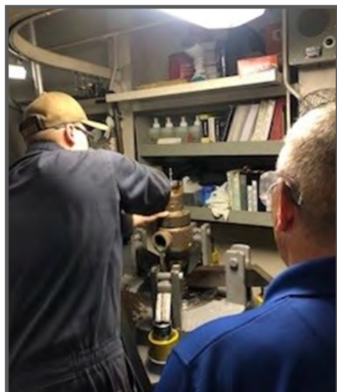
Mike Dengate from the NAMTS Afloat Team gives over the shoulder mentorship to HT2 Alex Weaver from Atlanta, GA, on how to adjust the pressure while pop testing a relief valve. (Photo by HTC(SW) Mike Vasquez.)
