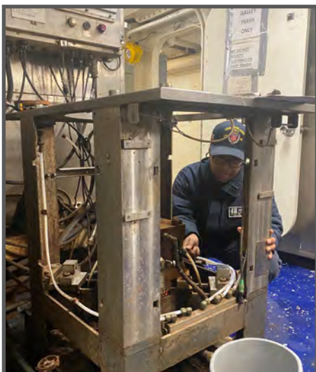
MM1(SW/AW) Rajah Stutts from Troy, Michigan, disassembles Nr. 1 Plastic Compress Melt Unit components.
