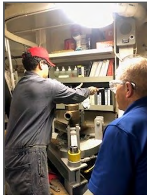
Mike Dengate from the NAMTS Afloat Team gives over the shoulder mentorship to HT2 Gabriel Gainey from Seattle, WA, on how to adjust the pressure while pop testing a relief valve. (Photo by HTC(SW) Mike Vasquez.)
