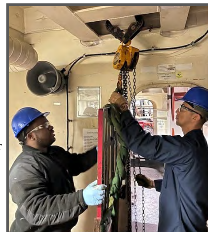
Aboard USS Carter Hall (LSD 50), BM2 (SW) Nelson Smith (left) and BM2 (SW) Ronaldo Beristain conduct a through ships rigging to satisfy line items on the Rigger Weight Tester JQR.
