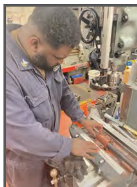
MR2 Michael Walker installs a piece of keyway stock on a tagged out milling machine aboard USS Carney (DDG 64). (Photo by Rick Smith).
