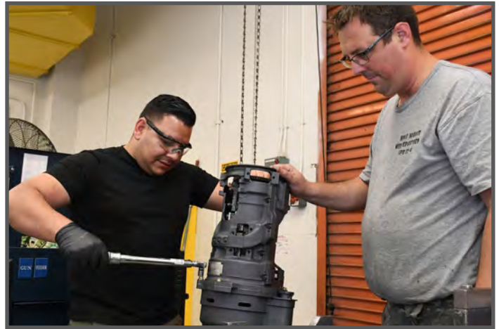
SAN DIEGO – Enrique Huanaco from Southwest Regional Maintenance Center's Ordnance Shop torques bolts on a 20MM Close-in Weapon System housing unit while an Australian Sailor from HMAS Brisbane (DDG 41) assists. While in San Diego last fall, Brisbane completed an availability while the crew engaged in interchangeability efforts at SWRMC. (U.S. Navy photo by Mr. Christopher Menzie/Released.)
