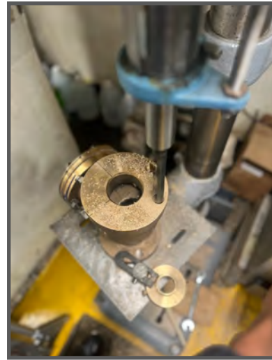
MR2(SW) Nathaniel Terry drills a 5/8 inch hole on a six bolt hole flange.
