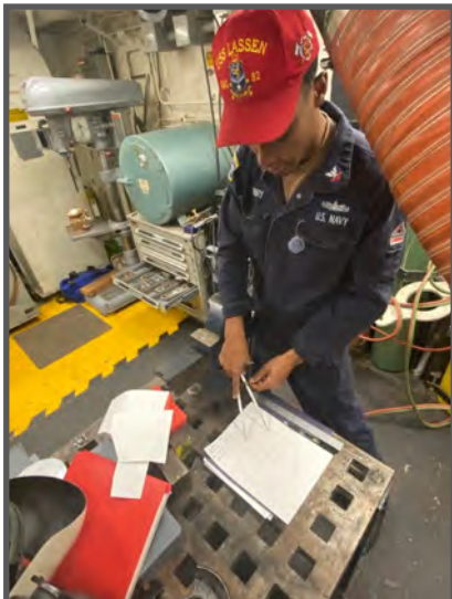
MR2(SW) Nathaniel Terry performs layout indexing for a six bolt hole flange aboard USS Lassen (DDG 82).
