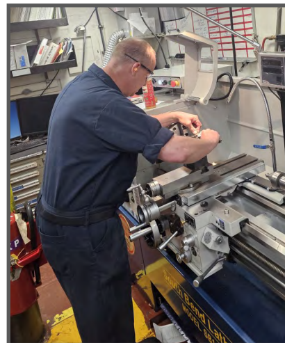
HT1(SW) Christopher Dreiling learns how to measure distance and read a dial vernier caliper. (Photo by DCFN Julian Gavazzi.)
