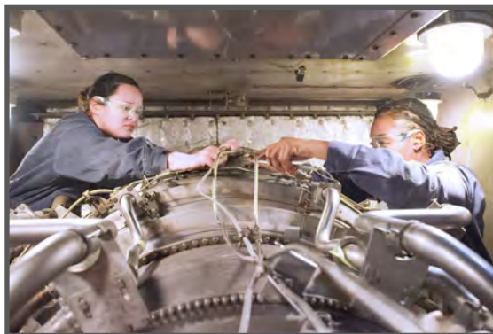
250327-N-GC612-1026, PEARL HARBOR, Hawaii (March 27, 2025) – Gas Turbine Systems Technicians (Mechanical) 1st Class Sharlyn Yambogonzalez, left, and 2nd Class Tabora Leach install fuel lines to a gas turbine engine on board Arleigh Burke-class guided-missile destroyer USS Hopper (DDG 70). (U.S. Navy photo by Mike Wilson)
