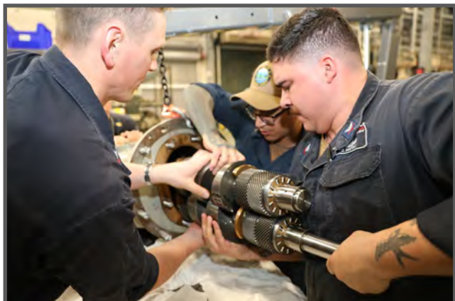
MM1 (SW) Samuel Wallace, MM2 (SW) Dominic Martinez, MM2 (SW) Joel Garcia are disassembling the ship-to-shop attached lube oil pump. (Photo by MM2 (SW/AW) Bianca Reiter.)
